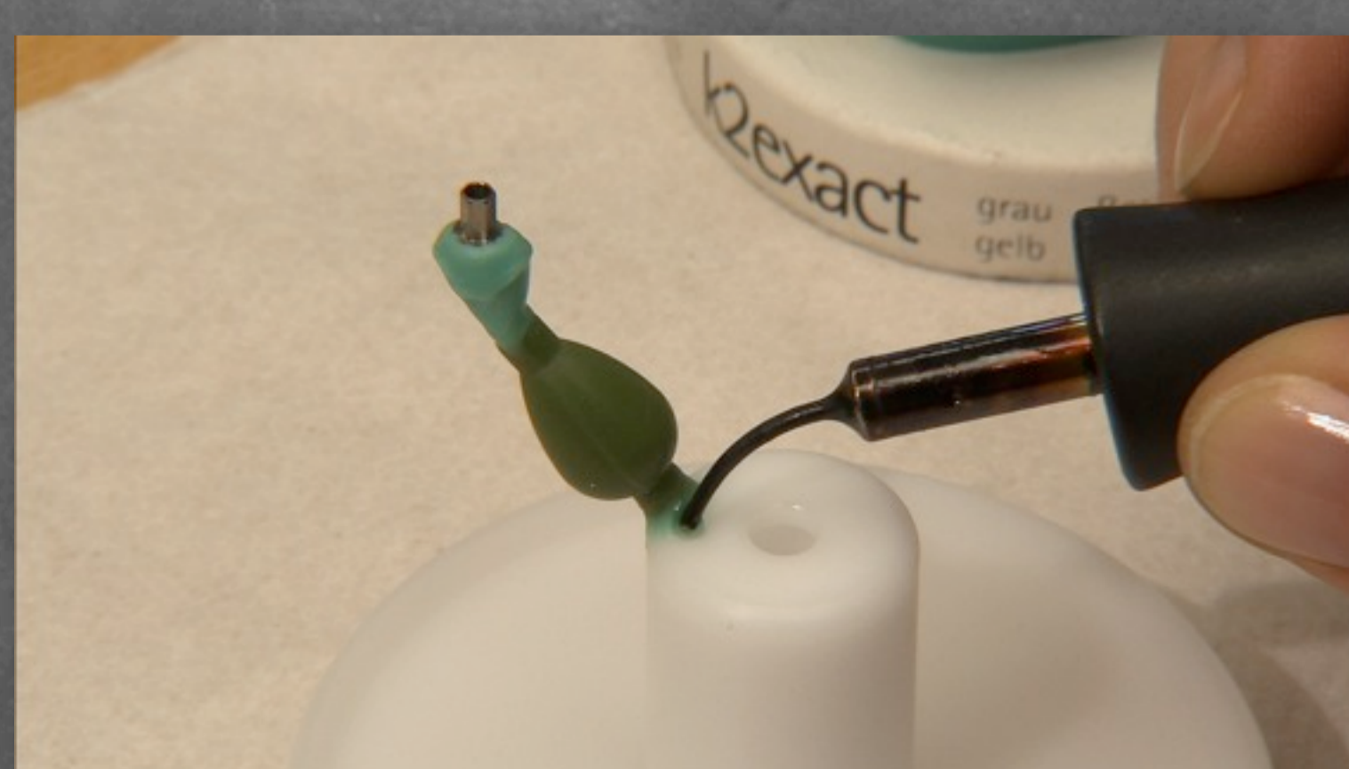
Fig. 3: Spruing the titanium-base/wax-up abutment.
